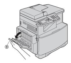
3. When the document has jammed near the roller: Hold the automatic duplex unit cover and remove the jammed paper (⑩) carefully by pulling it upward.
